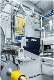
Fig. 2: Everything in a single working step: the input material goes from the MPR into the extrusion system and is then processed directly to make an inline sheet product. Photocredit: EREMA, Humer / Wallmen
