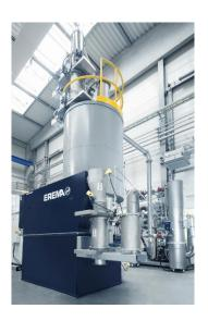
Fig. 3: The MPR from EREMA allows the decontamination, drying, dedusting and crystallisation of different PET input materials already prior to extrusion. Photocredit: EREMA, Humer / Wallmen
