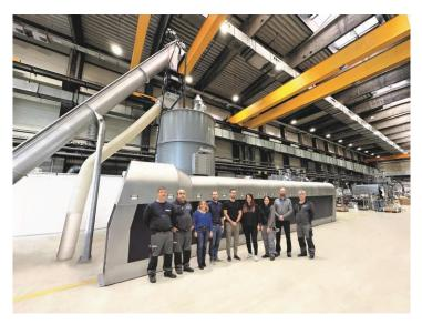
The INTAREMA® 2325 T-VEplus® RegrindPro® is the largest machine ever built for PO regrind and achieves a throughput of over 4 tonnes per hour. The picture shows the project team in front of the new plant.
